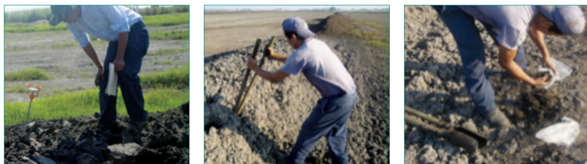
Fig. 5-7: Temperature is recorded and samples taken for moisture analysis.
