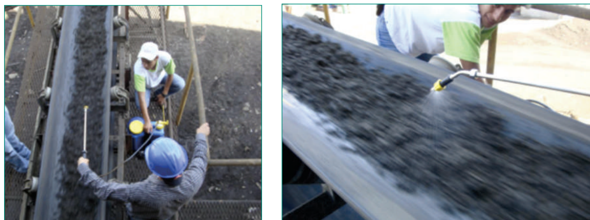
Fig. 3 & 4: The standard procedure of adding moisture to the cachaza before composting offered an ideal opportunity for seeding the cachaza with MICROBE-LIFT®
